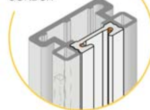
FL2 PROFILE with ELECTRIFIED CONDUIT
