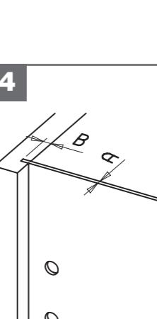
Presence and thickness of the back panel (A), depth of the milling (B).
