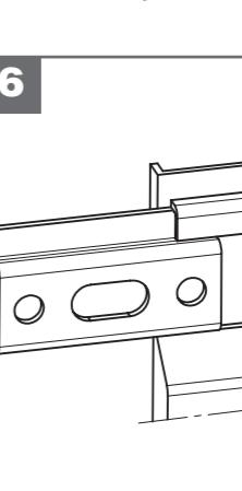
If the bracket is only partially hooked onto the wall plate.
