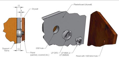
The Fastmount<sup>®</sup> multi-award winning system has revolutionized the mounting of panels. Panels can easily be removed and refitted in any sequence time after time. For further information or technical support contact: info@fastmount.com
