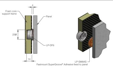
The Fastmount® multi-award winning system has revolutionized the mounting of panels. Panels can easily be removed and refitted in any sequence time after time. For further information or technical support contact: info@fastmount.com
