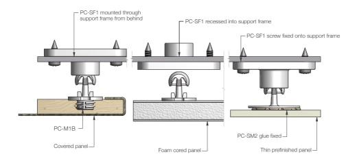
The Fastmount® multi-award winning system has revolutionized the mounting of panels. Panels can easily be removed and refitted in any sequence time after time. For further information or technical support contact: info@fastmount.com
